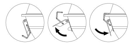
To unlock lid: lift up lock handle, remove lock bracket from lid, push lock handle down.
